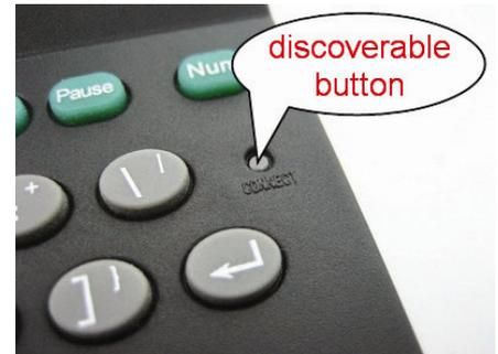
6, Begin a device detection on PC, Phone or PDA, and locate the mini bluetooth keyboard among any found devices.
